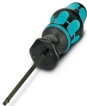
Torque screw driver with preset torque of 0.8 Nm, with 4 mm hexagon for accommodating SAC bits, two-component handle with non-slip grip
